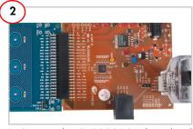
1. Connect the CY3280-BSM board to the CY3280-20x34 UCC board's P2 connector.
