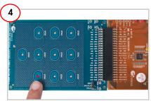
1. When you touch a button, the corresponding LED on the module board lights up, indicating the button you touched.
